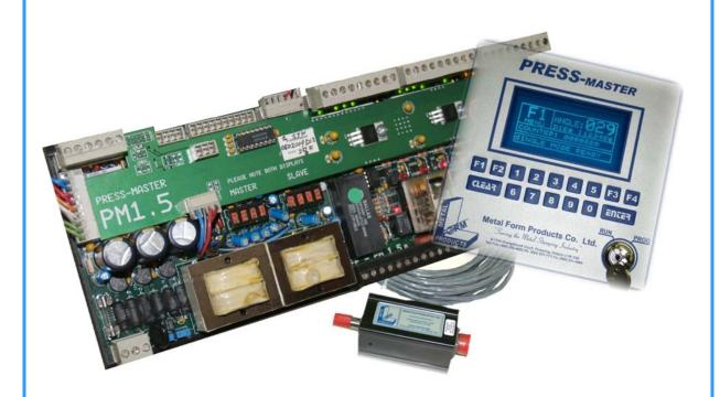
The PressMaster PM 1.5 is a control-reliable clutch / brake system that uses state of the art technology to incorporate press automation features such as Die Protection, Programmable Cams, Tonnage Inputs, (strain gauges extra), Job Memory, Job Counters and a Time-Based Brake Monitor.
